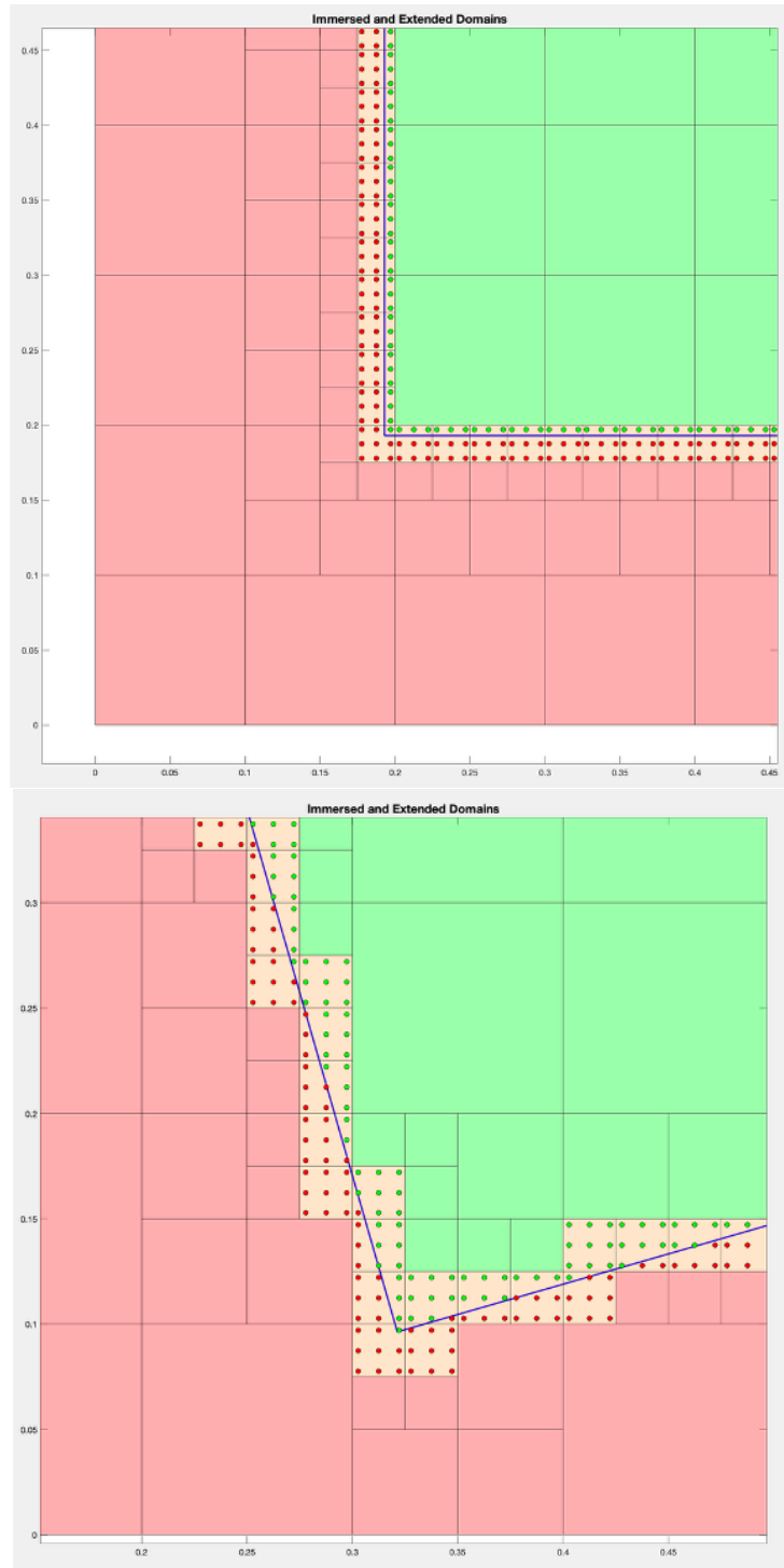
Figure 10: Controlled comparison of two immersed-square configurations integrated with a three-level quadtree, identical in square, polynomial degree, number of elements and quadtree depth, and with a tiny cut cell of identical mass by construction. (a, b) Axis-aligned square and a detail at a cut cell; (c, d) the same square rotated and a detail at a cut cell. The physical domain (green) is immersed in the extended domain (pink); cut cells along the boundary are refined by the quadtree, and quadrature points are classified as interior (green) or exterior (red). Largest discrete frequency and critical time step: aligned \omega_{\max} = 1.23 \times 10^3 , \Delta t_{\text{crit}} = 1.463 \times 10^{-3} ; rotated \omega_{\max} = 8.63 \times 10^9 , \Delta t_{\text{crit}} = 2.085 \times 10^{-10} .
